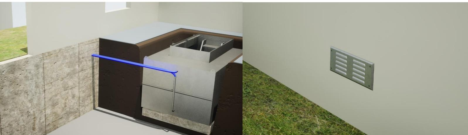
The ventilation hoses are connected to the dedicated openings in the wine cellar and led all the way out to an exterior wall. Here they are attached and hidden behind the ventilation grill that comes with the wine cellar. The purpose of the ventilation hoses is to ensure that the air in the wine cellar is constantly replaced. The wine cellar uses passive cooling and ventilation without the use of energy. Thus, it is neither a burden on the environment nor the electricity bill.
