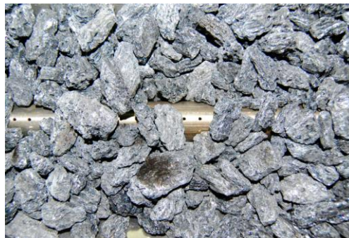
Photo 2 – Decorative stones location on burner
